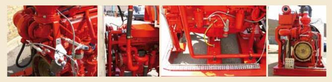
Compliant as a component to ATEX 94/9/EC. Full ATEX upfit accessories available from Pyroban.
