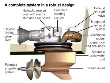
The Volvo Penta IPS has been developed and is manufactured as a complete system from the helm to the propeller cone – engine, propulsion unit incl. gear box, propellers, exhaust and seawater system, steering, and controls.
