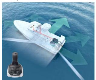
With the joystick the helmsman can now maneuver the vessel in any direction at low speed – with just one hand. The joystick is coupled to a sophisticated and specially developed software that individually commands the electronically engines and the pod units to steer, throttle and shift gears independently, making the boat move in any direction the driver wants – sideways, diagonally, forward, backward or rotate.
